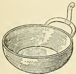
Fig. 19—Method of gating a cover for an electric drill
